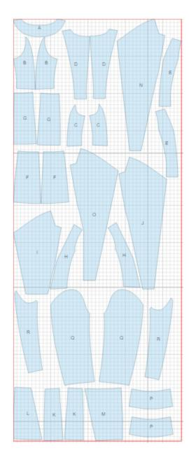
Note: lining for back and front are cut from the same pattern, excluding the width of back neck facing and front facings.
